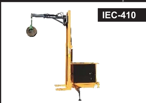
Hook Stacker Cap: 500/1000 kgs Lifting ht: 1600/2500/3500
